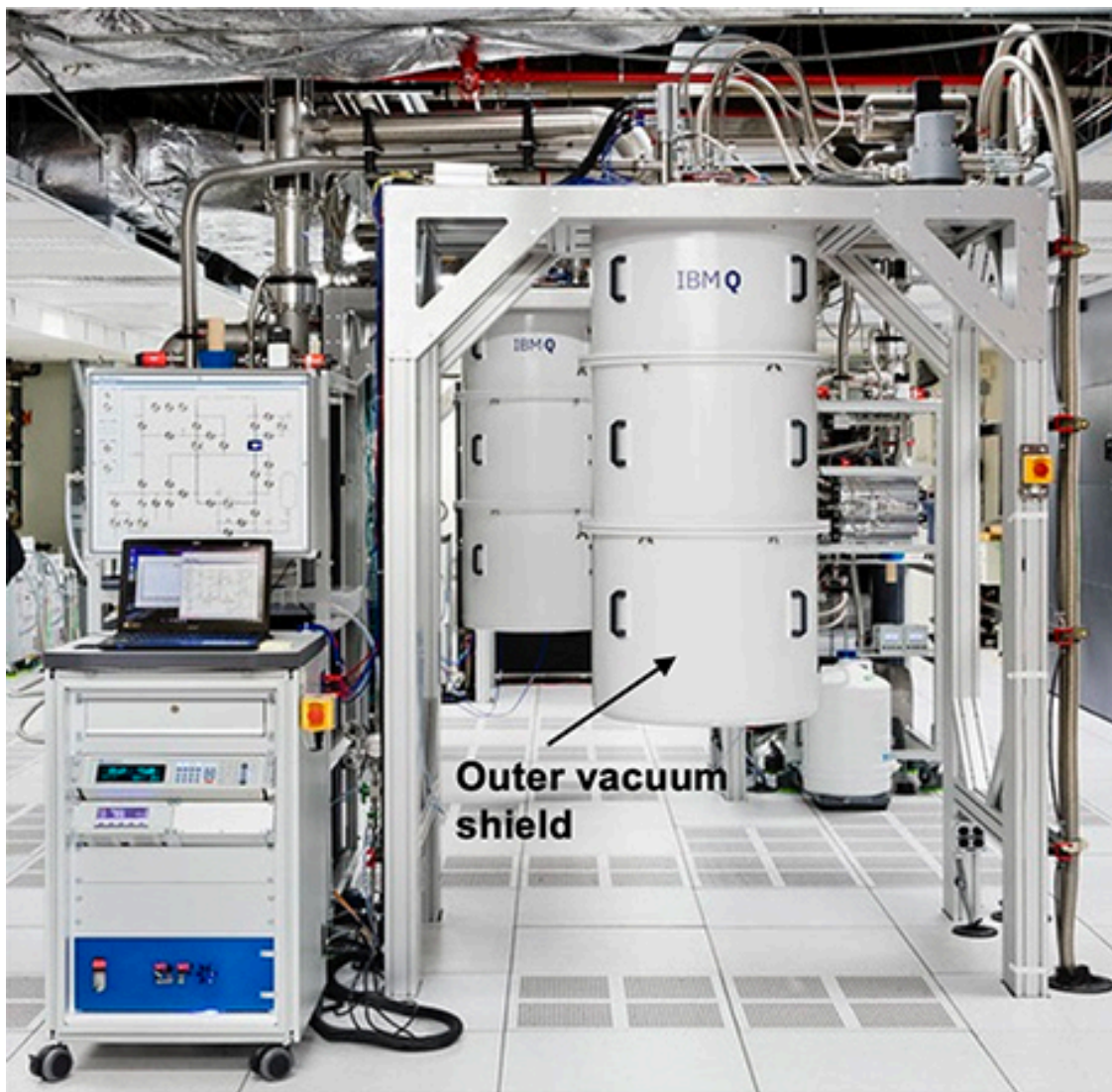
Dilution fridge setup: outside view
